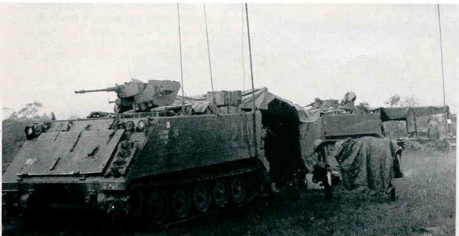
Shortages of M-577 Command Post Vehicles led to some M-113s being converted to Mobile Command Posts, with the designation M-113 MCP. Their configuration did not set them apart from other A.P.C.s as much as the M-577 did, thus making it harder for the enemy to pick them out. (US Army)
