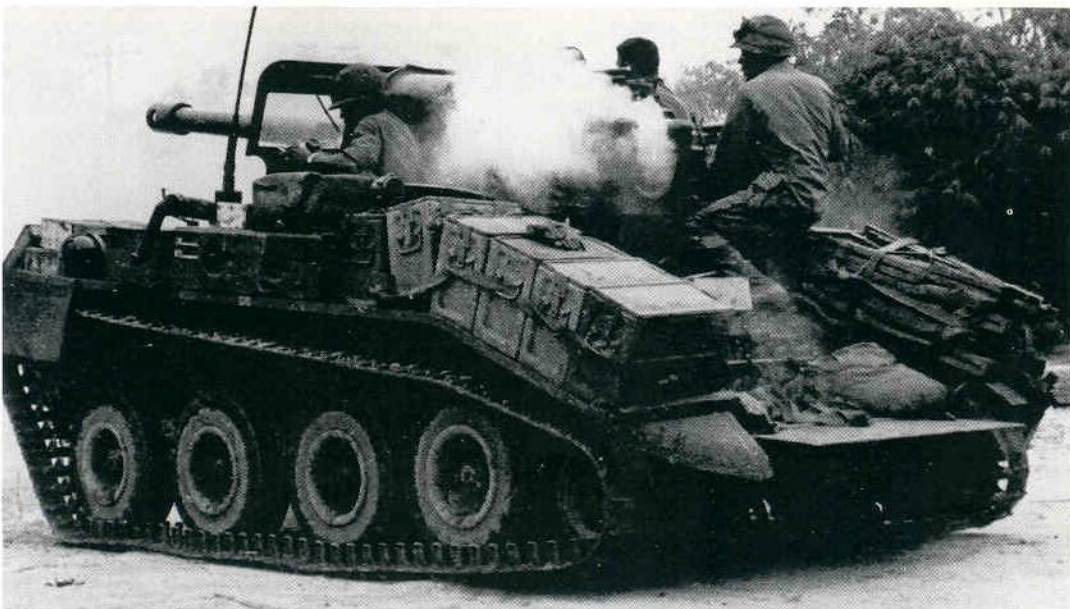
A Scorpion fires on a V.C. force during an attack on a convoy. A serious drawback of the M56 was the exposed conditions of the crew. (US Army)
