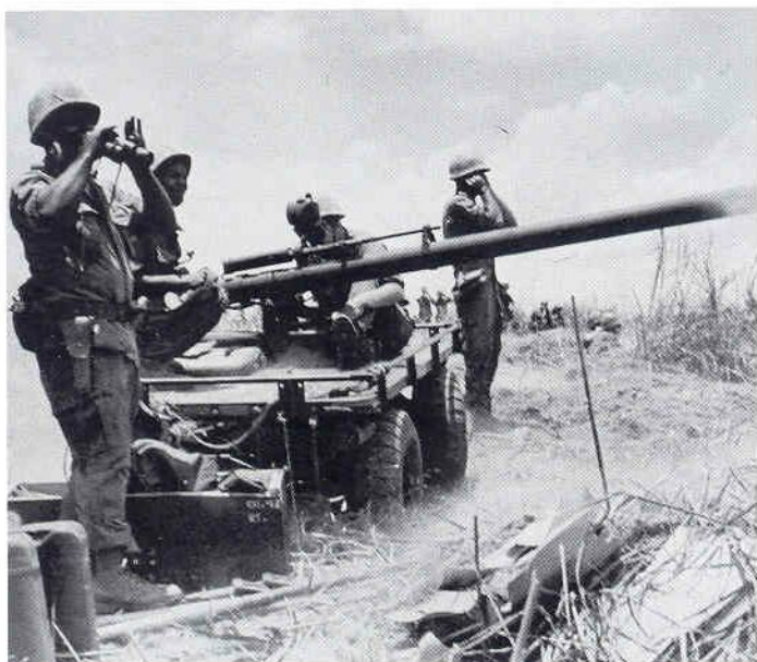
(Above) 106mm recoilless rifle, mounted on a M-274 mechanical mule, fire on enemy positions near Khe Sanh. These lightweight vehicles were often helicoptered in to provide marines with a small mobile support weapon. (USMC)
