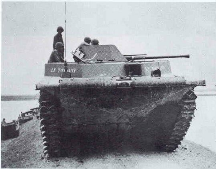
Crab (weasel) prepares to go on an operation in northern Vietnam. It was standard procedure to raise the forward shield for improved visibility of the low seated driver. (Balin/E.C.P.)
