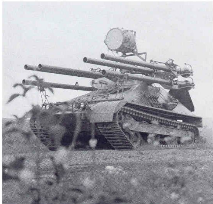
Unusually modified Ontos carries a large searchlight for night firing. Very few vehicles of this type were so equipped. (USMC)
