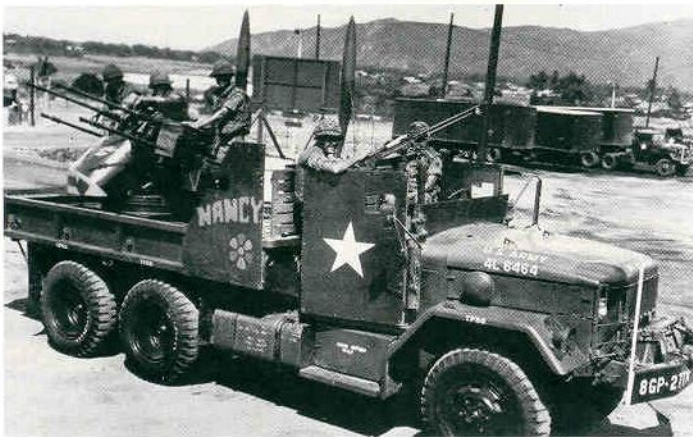
Nancy, a M-35 2½ ton truck equipped with a quad fifty and partial armor for the cab. M-60 mount in cab provided close-in security for quad crew. (US Army)
