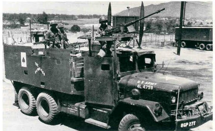
The Gamblers, another M35 is outfitted with full armor and a variety of machine guns. Even when modified as this, the crews were still exposed since the weapons needed an adequate field of fire. (US Army)
