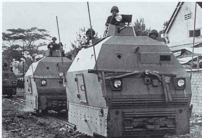
Self-propelled railroad armored cars, called Wickums , were used, along with armored trains, to keep the rail lines opened. They proved unable to cope with the elusive Viet Cong forces. (U.S. Army)
