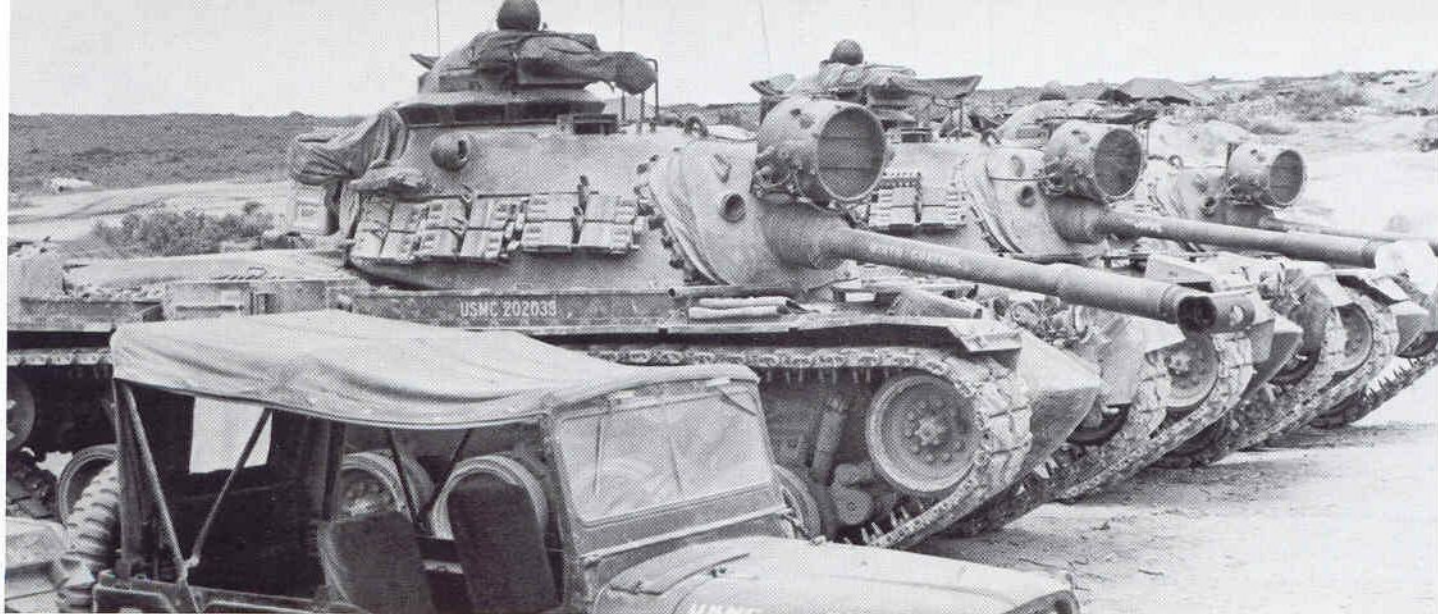
Three Pattons from the 3rd Tank Battalion at a base camp north of Hue. The first two have had their cupolas modified with an additional section to increase visibility. (USMC)
