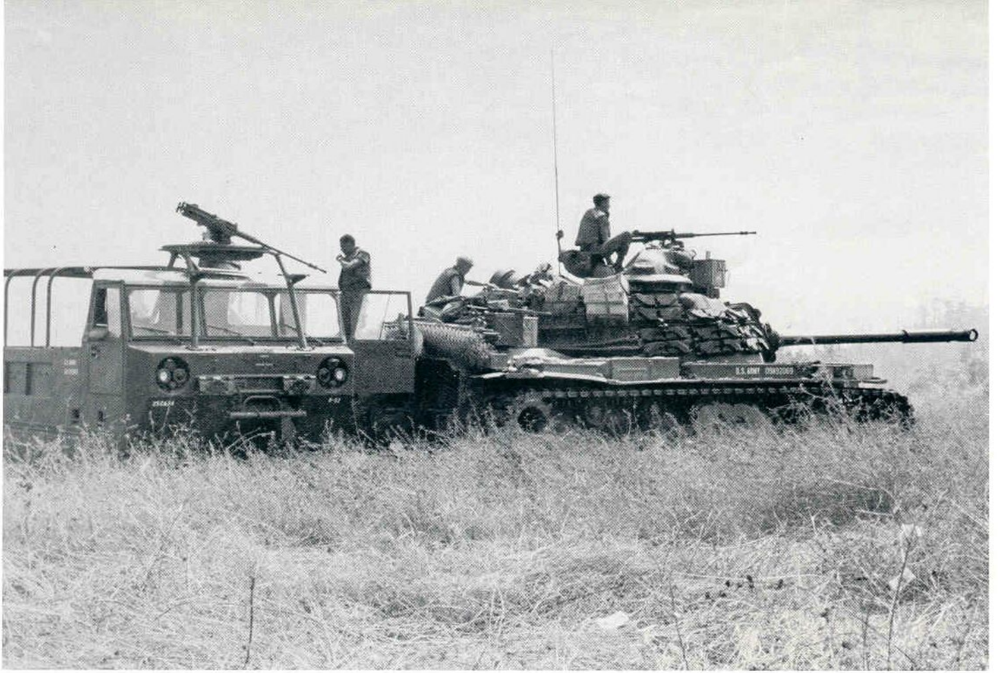
(Above) An M-48 being resupplied by an M-548 cargo carrier near the Black Virgin Mountains, a notorious V.C./N.V.A. stronghold. The M-548 was derived from the M-113 and provided good cross-country supply capabilities to field units. (US Army)
