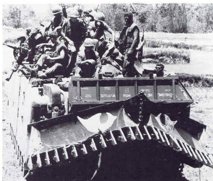
(Above) Fierce looking LVTE, loaded with marines, moves across a rice paddy. It appears to have some sort of container wedged behind the plow. (USMC)
