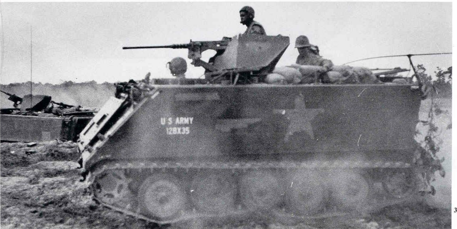
Early U.S. vehicles had numerous White markings which the enemy used for aiming points. Troops soon painted them over or in the case of this M-113 used Olive Drab tape to cover the star and some lettering. (US Army)
