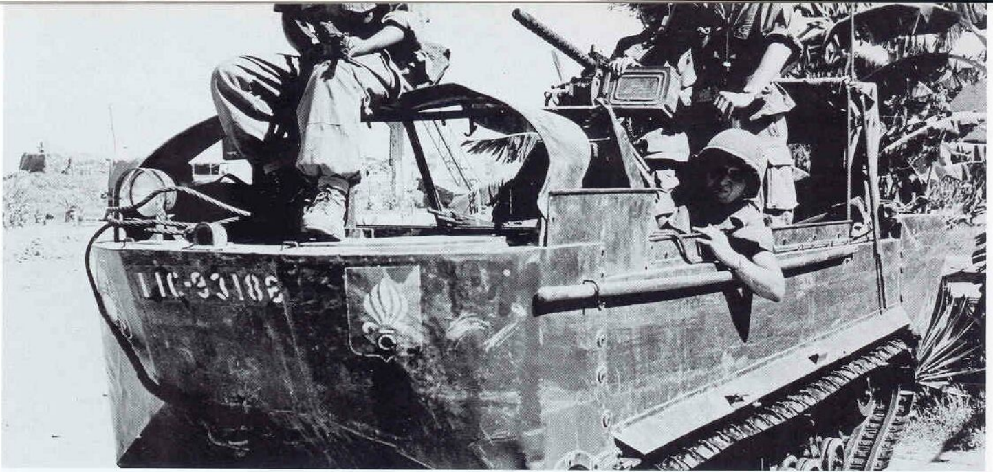
Crab (weasel) prepares to go on an operation in northern Vietnam. It was standard procedure to raise the forward shield for improved visibility of the low seated driver. (Balin/E.C.P.)
