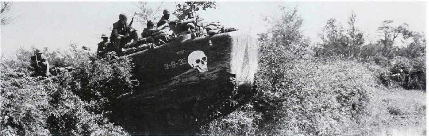
(Above) Interestingly marked LVTP-5 crashes through a hedgerow south of Danang. Troops preferred to ride outside because if a mine detonated, the fuel tanks would often rupture and incinerate those inside. (USMC)
