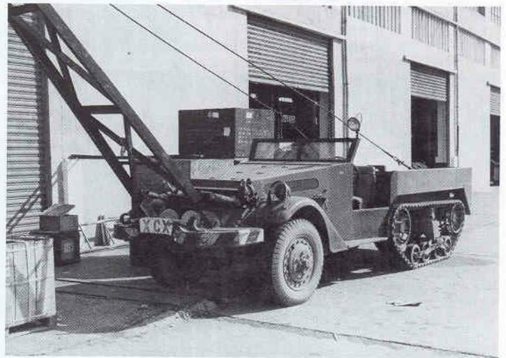
Modified ARVN halftrack as a wreck and barrier removal vehicle. (U.S. Army)
