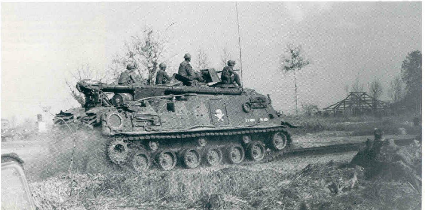
(Below) M-88 moves out from base camp with an armored unit. These vehicles were in constant demand to help keep tanks and APCs in running order and often accompanied units on missions in the field. (Papson)
