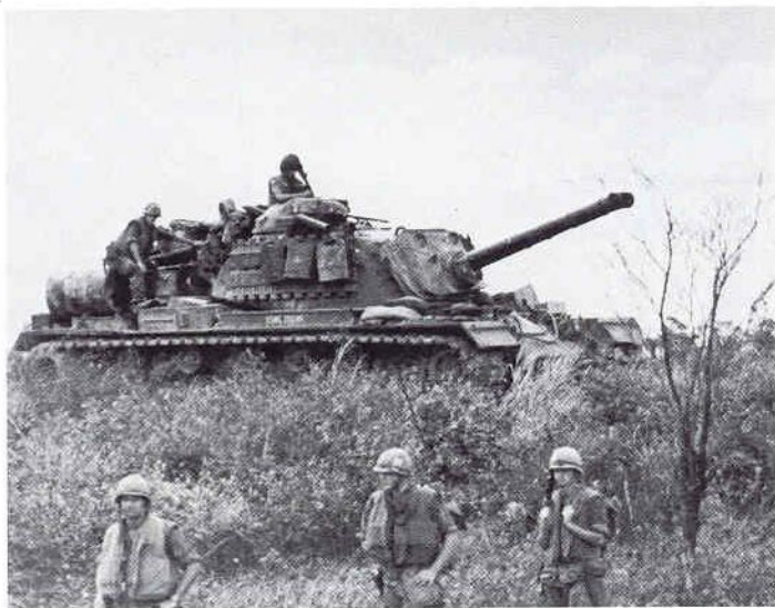
(Above) M-67, heavily loaded, cover marines during OPERATION HICKERY II. Extra treads on turret provided protection from enemy anti-tank weapons. (USMC)
