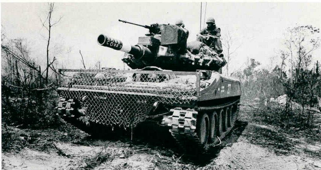
An M-551 Sheridan from the 4th Cavalry on patrol with elements of the 25th Infantry Division. Wire screen is fitted to keep vegetation out of the drivers way. (US Army)
