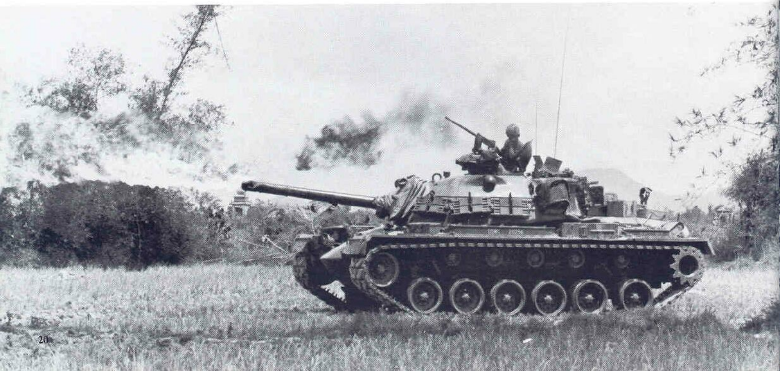
Flamethrower tank in action south of Da Nang. Nicknamed Zippos , they were never used extensively because of the availability of napalm from marine aircraft. (USMC)
