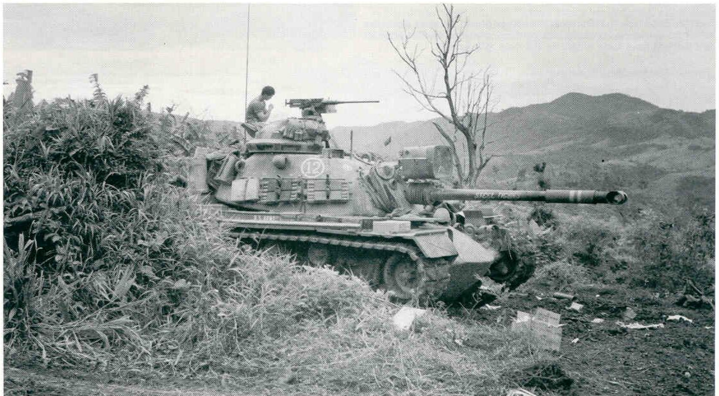
This M-48, from the 5th Infantry Division (Mechanized) awaits orders to move out during OPERATION UTAH MESA in the Khe Sanh area. Often the cupola machine gun was mounted outside for easier handling and a better field of fire. (US Army)
