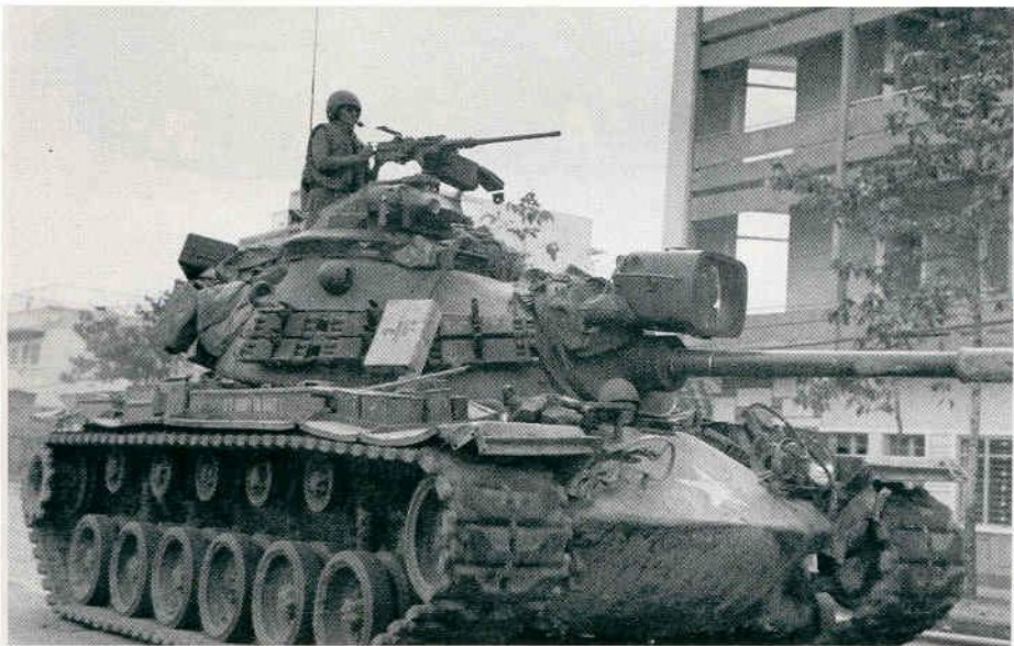
M-48 of the 4th Cavalry, 25th Infantry Division, provides fire support for ARVN Rangers in Saigon during the Tet offensive. Cupola has been fitted with a vision block ring to increase visibility. (US Army)
