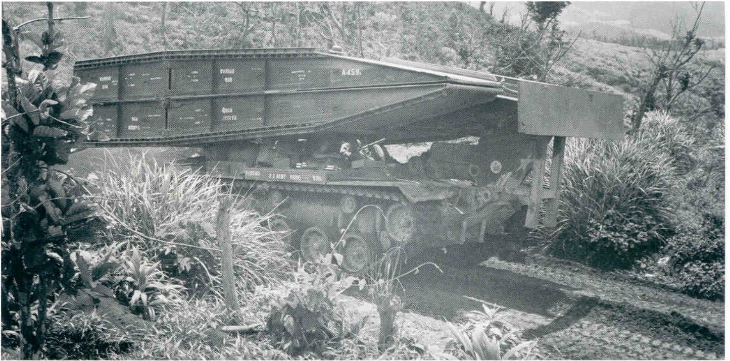
AVLB bridge layer on an M 60 chassis en route to a new base camp during OPERATION UTAH in the Khe Sanh Area. Both M48 and M60 AVLBs were used in Vietnam. (US Army)
