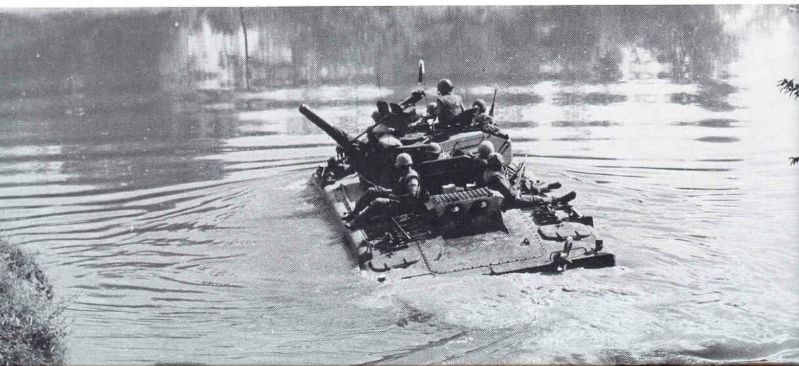
LVTH ferries marines across a river during a search and destroy south of Da Nang. Vehicle is armed with a 105mm howitzer. (USMC)
