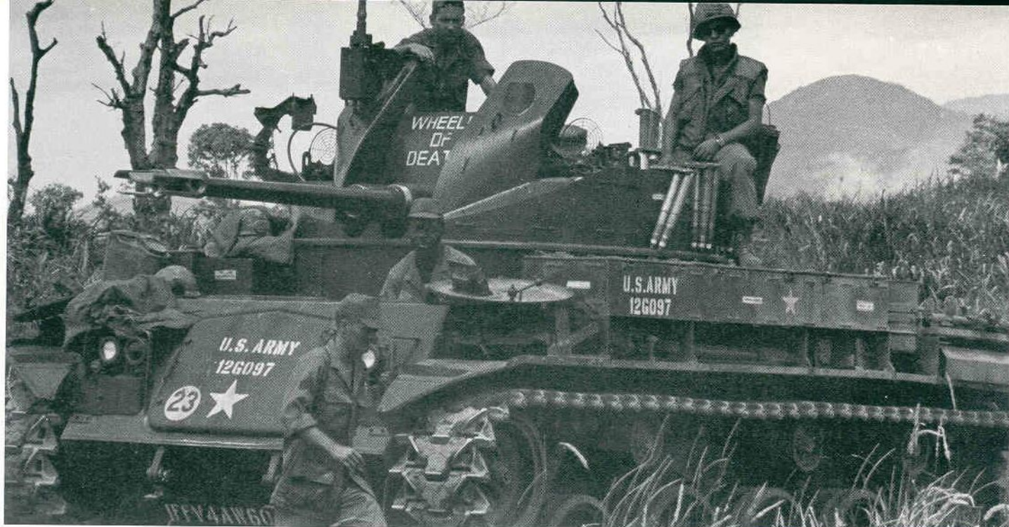
Wheels of Death , an M42A1 Duster assigned to II Field Forces, prepares to move out to a new position. One crewman wears a flak jacket in case of enemy fire into his exposed position. Clips of 40mm ammunition are positioned on turret for easy access. (US Army)
