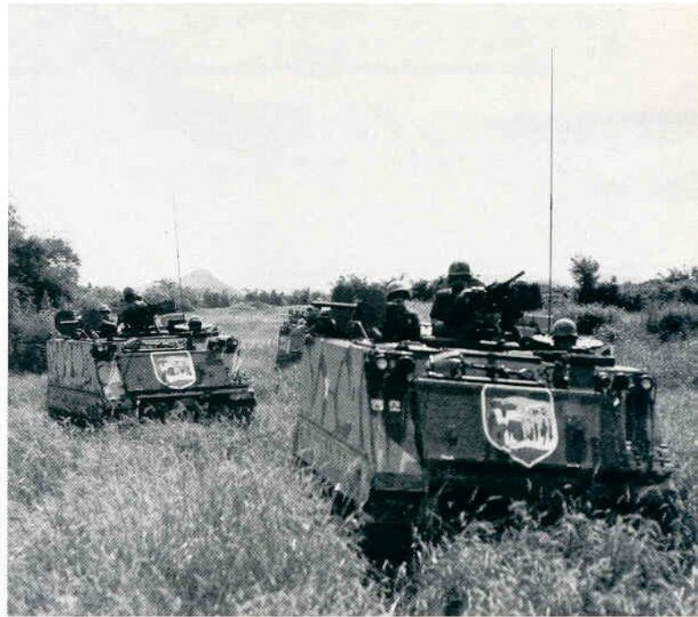
M113s of the Korean Tiger Division move through the brush near Qui Nhon. APCs are camouflaged with a Sand-Tan over Olive Drab while tiger is Orange, Black and White on a Red shield. Note unusual shape to shields in rear. (US Army)
