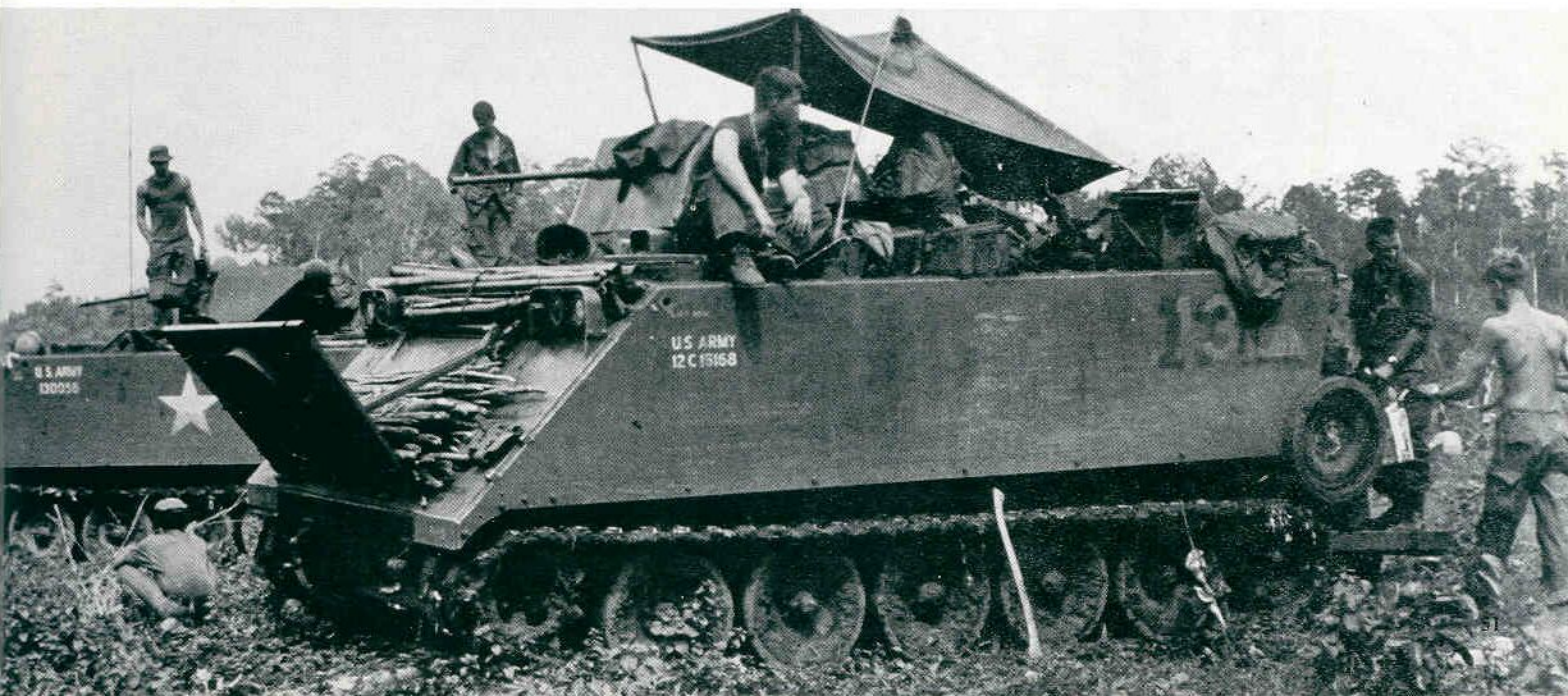
A.P.C. crews from the 10th Cavalry take a break during a search and destroy mission. Wood bundles on front of hull were useful for traction if the vehicle became bogged down. (US Army)
