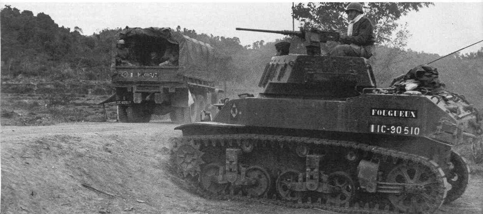
An M-8 Howitzer Motor Carriage (H.M.C.) helps provide convoy security in the Tonkin area. Note mixture of bogey wheel types and the rubber block type track. (Balin/E.C.P.)
