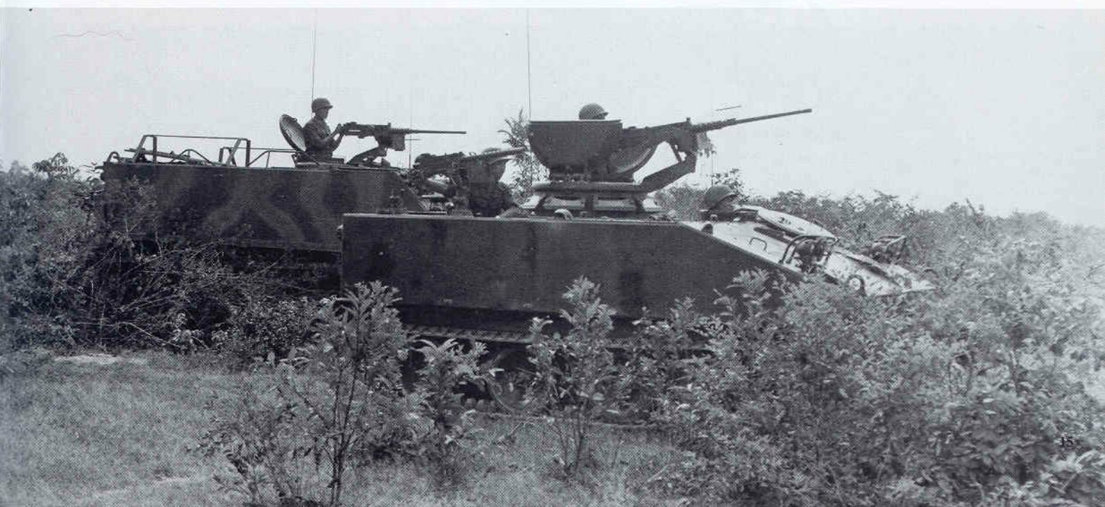
ARVN M-114, with M-113 in background, maneuver during training. The M-114 proved to be totally unsuited for use in Vietnam and was quickly phased out. (U.S. Army)
