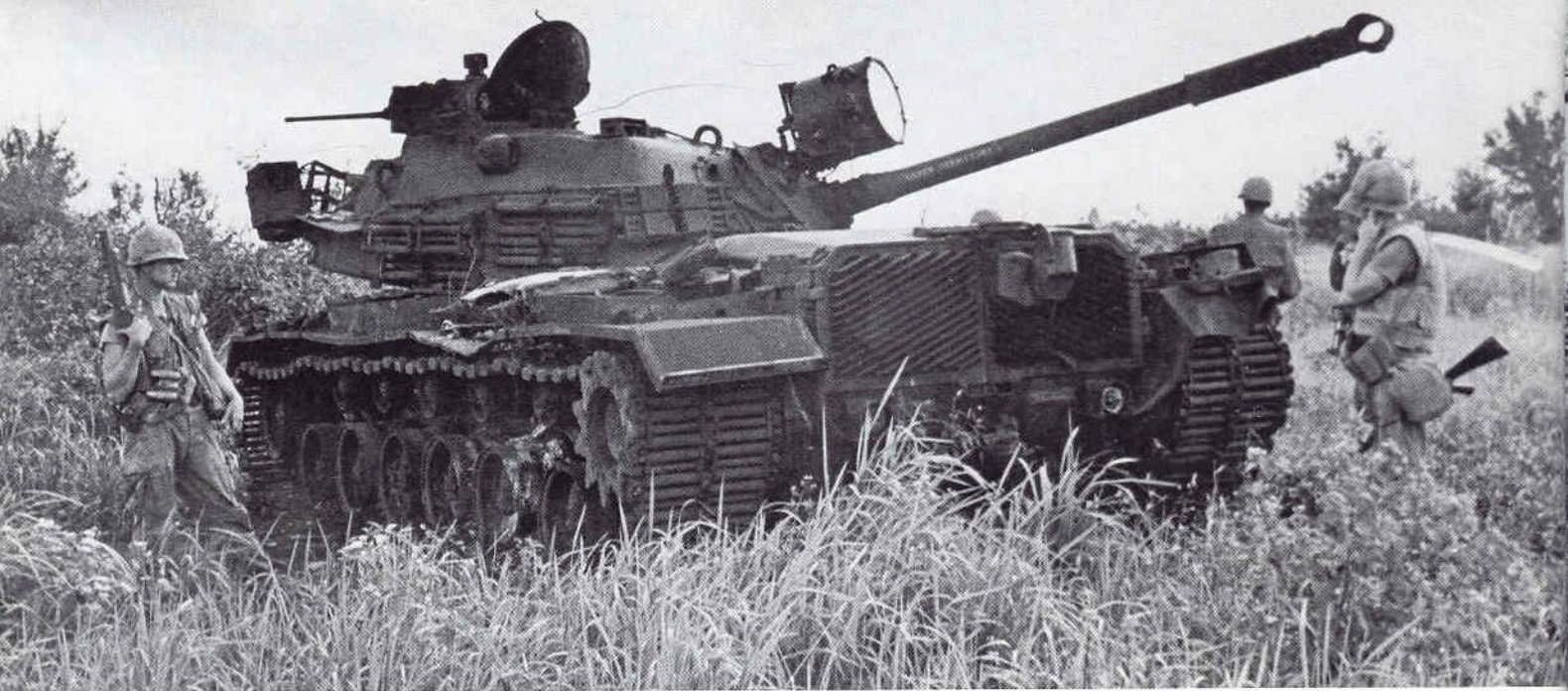
(Below) Sandbagged Ontos moves towards a new position during OPERATION IOWA. Note raised slats on sides to help carry more gear and the use of vegetation to break up the vehicles outline. (USMC)
