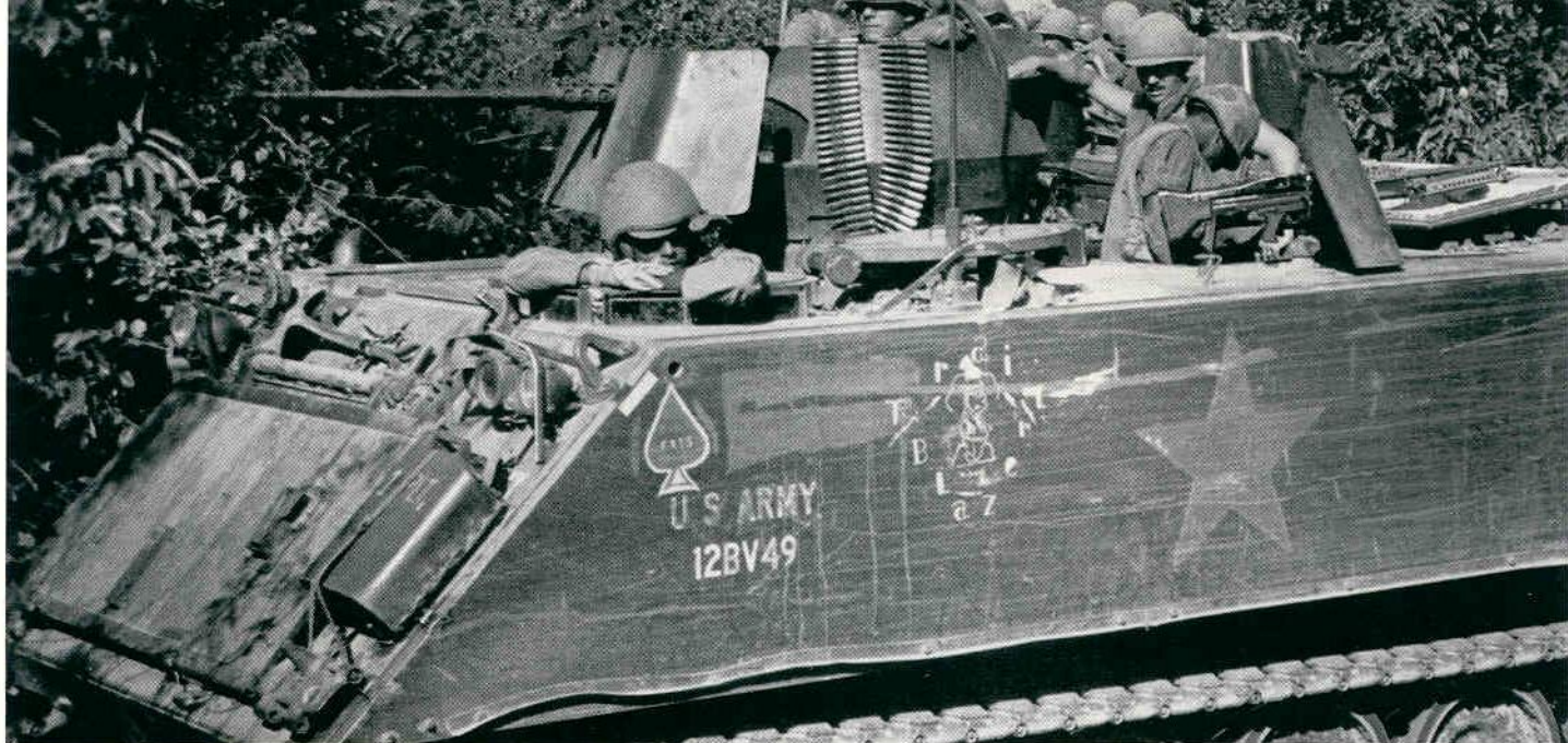
M-113 ACAV fitted with additional shields and machine guns. Note how star is painted out, and the spade insignia on hull. Nicknamed Trailblazer it is from the 11th Cavalry. (US Army)
