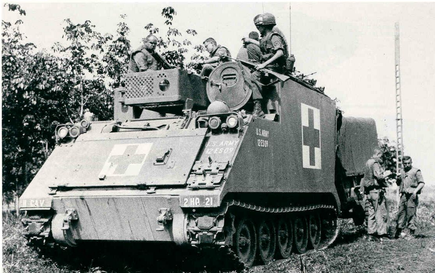
M-577A1, fitted as a mobile aid station, from the Headquarters Troop of the 11th Cavalry. Vehicle is participating in a search and destroy mission near Xuan Loc, east of Saigon. (US Army)
