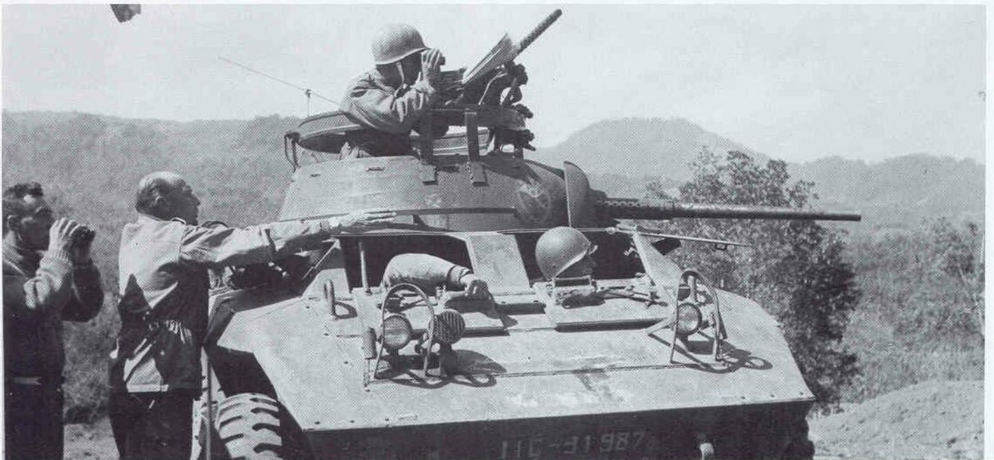
Unit commander directs M-8's fire during fighting at the Noire River, January 1952. Fenders were often removed due to battle damage or because they collected large quantities of mud. (Balin/E.C.P.)
