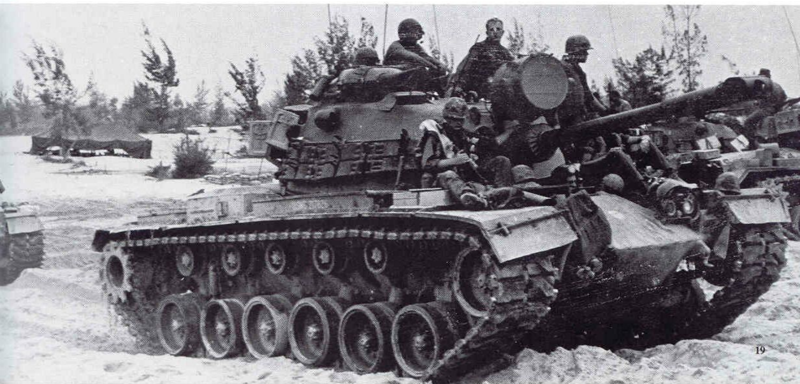
During OPERATION ARCADIA, M-48s move through heavy sand in support of the 1st Battalion, 1st Marine. Turret mounted searchlights proved invaluable during night fire fights. (USMC)
