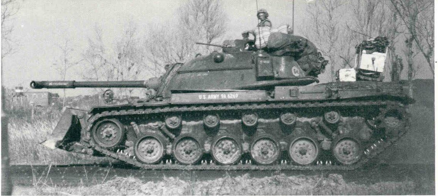
An M-48 equipped with an M-8A1 dozer blade moves down a road during a search mission. Note how the tank's suspension is compressed in front from the dozers weight, and the numerous personal effects of the crew, including a mattress on the turret. (Papson)
