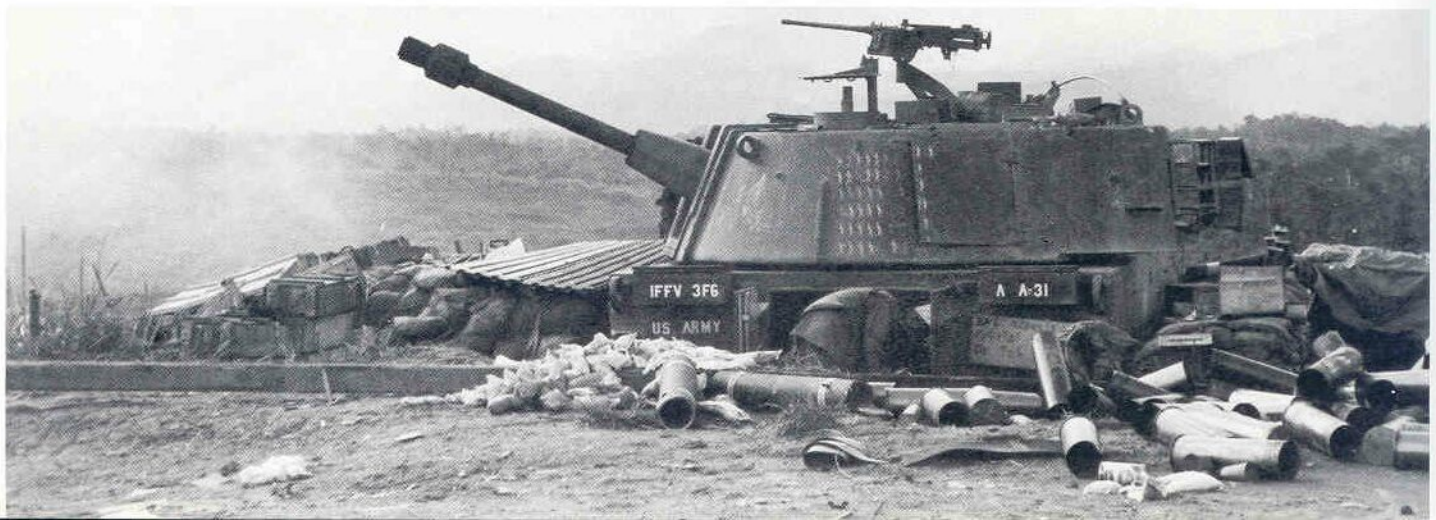
M 108 S.P., from the 52nd Artillery Group, 6th Artillery, in a bunkered position. Note kill tally on side of turret. The vehicle mounted a 105mm howitzer. (US Army)
