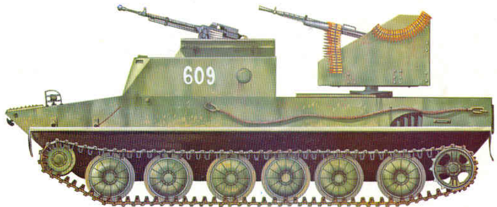
NVA BTR 50P with A.A. gun turret on rear deck, captured at My Chanh in May, 1973.
