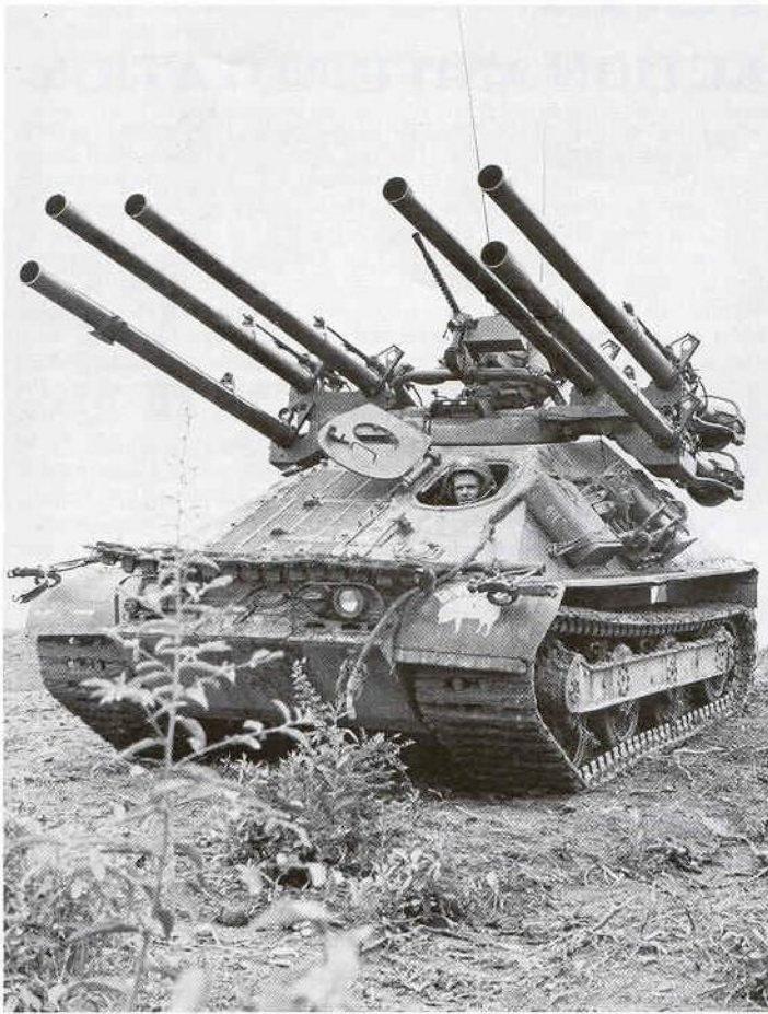
An Ontos, with its guns at full elevation to increase their range, prepares to fire during OPERATION MOBILE, near Chu Lai. Note the unusual artwork on the fender, rarely seen on the Ontos. Closest jerrycan is marked on its side so as not to be contaminated with gas or water. (USMC)
