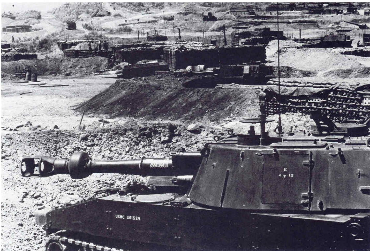
Assassin , one of the 155mm M-109s from K Company, 3rd Battalion, 2nd Marine await fire support call. Part of the unit's designation can be made out on the turret door. (USMC)
