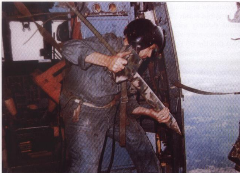
Airborne-delivered sensors played a key role in the defense of Khe Sanh, here an Air-Delivered Seismic Intrusion Detector (ADSID). There were several versions, and could detect the vibration of troops moving (seismic) or be activated by the sound of voices and movement (acoustic). Monitoring stations picked up the signal, and the general area in which the sensor had been planted was saturated by artillery and air strikes.
