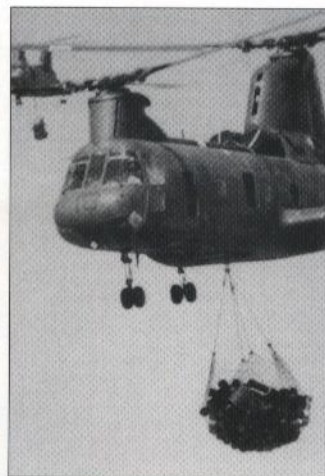
A Super Gaggle flight of CH-46A "Purple Foxes" make a run into a hilltop position. The netted cargo sling would hit the ground, the crew chief would immediately release the cargo hook, and the chopper lift off in seconds. This sling load carries plastic-lined, steel 155mm propellant tubes filled with water. The tubes were plentiful and survived dropping from a low height.
