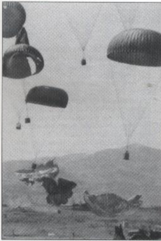
G-12 64ft diameter cargo parachutes descend on the Khe Sanh DZ, each carrying up to a ton of supplies or ammunition. The airdrops were extremely accurate and few missed the 200 x 300m DZ. Recovery crews are already moving out.
