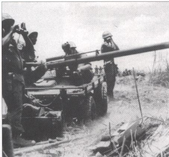
A Marine battalion had eight 106mm M40A1 recoilless rifle mounted on M274A1 "Mechanical Mule" 1/2ton weapons carriers. Fitted atop the 106mm is a .50-cal M8C spotting rifle, using different ammunition than the .50-cal machine gun. It allowed the gunner to accurately adjust his aim before firing the main gun. The "One-Oh-Six" was used for supporting and suppressive fire, countermortar, and countersniping.
