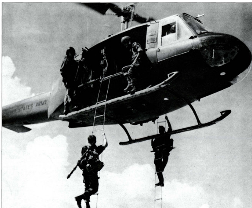
Reconnaissance troops climb 80ft. wire ladders with aluminum-tube rungs into a UH-1H Huey. These allowed reconnaissance teams to be extracted from pick-up zones on which helicopters could not touchdown. The ladders were carried rolled up on the skids and dropped with sandbags attached, to carry them through vegetation.
