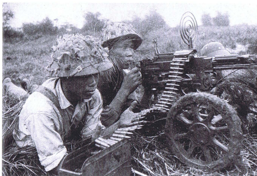
This 7.62mm SGM heavy machine gun crew have camouflaged their sun helmets with camouflage-pattern parachute fabric secured in the netting. The ammunition container held a 250-round, non-disintegrating, metallic link belt. The anti-aircraft ring sight is fitted to the gun, but this could also be used against ground targets.
