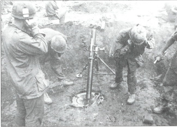
The 81mm M29A1 mortars normally remained in firebases for close-in defense and to support local security patrols. Besides HE and WP ammunition, they also fired parachute illumination flares, one of their most valuable uses.
