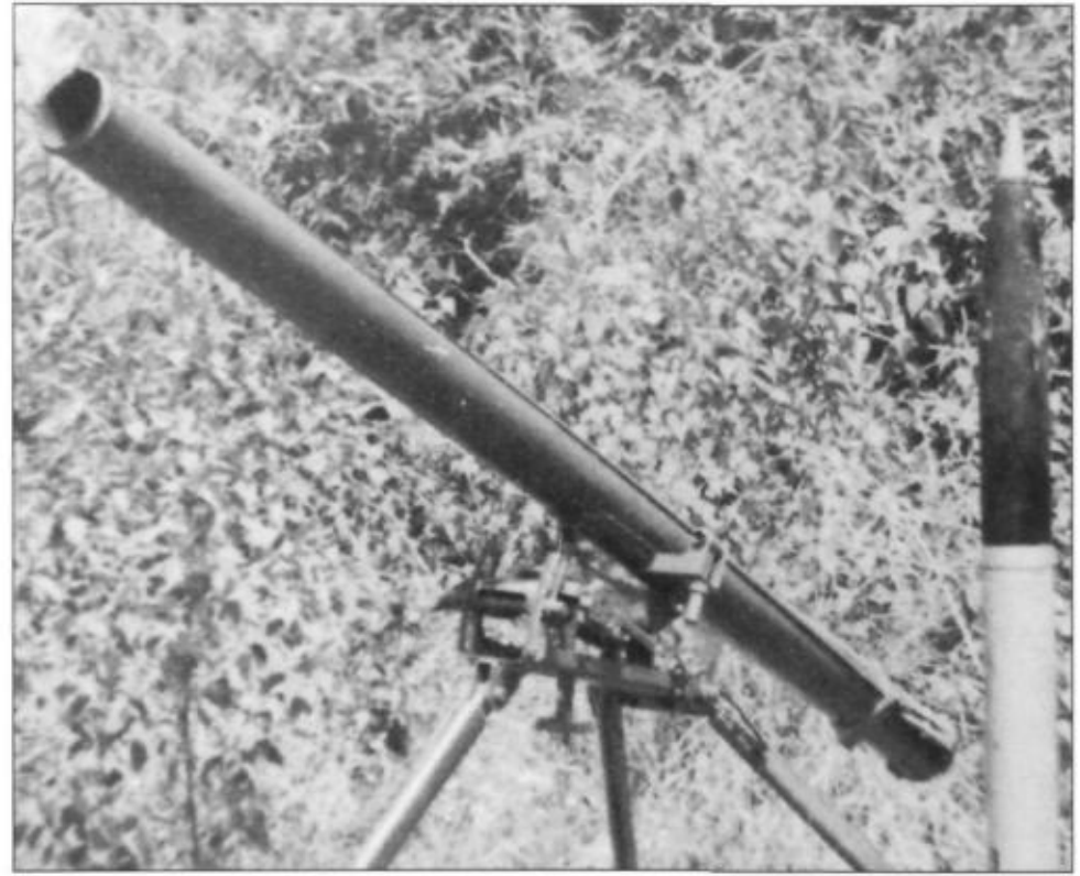
VC rocket artillery battalions were armed with the Soviet 122mm DKB. The launcher had an 11,000-yard (10,000m) range. It could be broken down into man-pack loads. Simple wooden launch troughs and even earth ramps were also used to launch the rockets.
