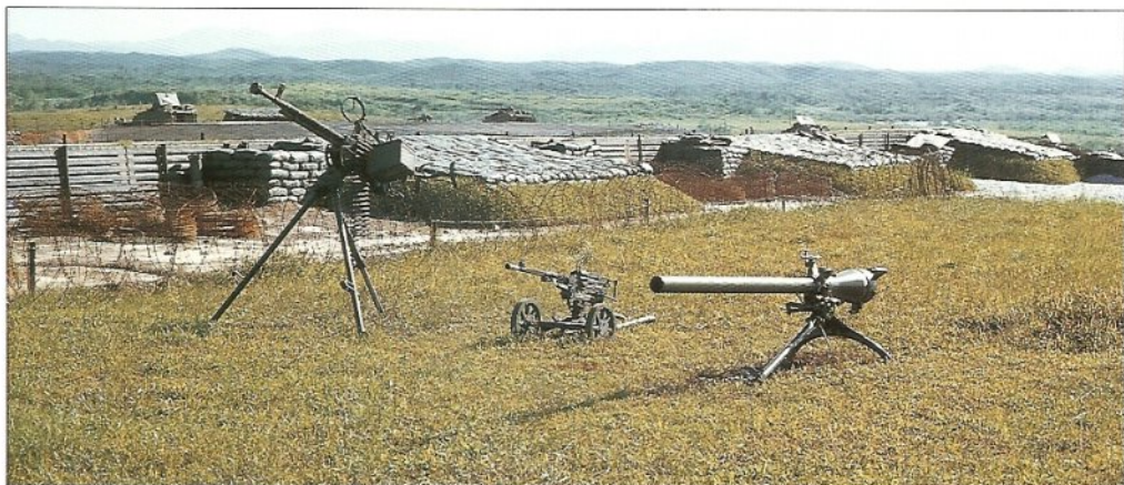
From left to right: a captured Soviet Degtyarev 12.7mm (.51-cal.) DShK38/46 (Chinese Type 54) AA machine gun; a Goryunov 7.62mm "heavy" (actually medium) machine gun (Chinese Type 57); and a Chinese 75mm Type 56 recoilless rifle (copy of US M20). As with all communist weapons used in Vietnam, the basic designs were manufactured in both the USSR and China, with slight differences in each case. The machine guns, especially the 12.7mm, were the weapons normally posing the most serious threat to Freeworld helicopter pilots when they flew near the ground in bandit country. (Don Aird)
