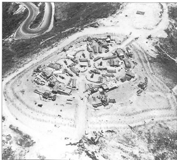
Aerial view of the USMC FSB Los Banos (Thua Thien province, on the coast near Da Nang) in April 1970. This firebase had first been occupied by 101st Airborne Division, then evacuated; then reoccupied by the Marines. It is almost a "model" for a company position built on a hilltop, enclosing a battery of M102 105mm howitzers and some mortars, including three lines of wire and anti-rocket wire mesh screens in front of major command bunkers. However, the gaps in the wire for the central road might be a defensive weakness unless they were regularly closed when the road was not in use. (US National Archives)
