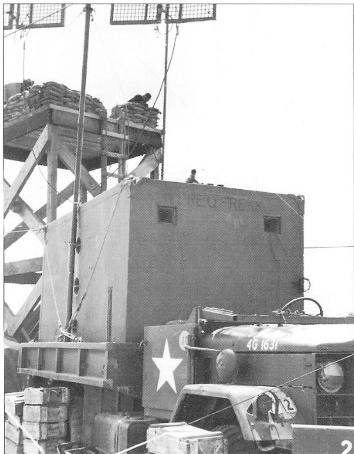
"Freq Freak" – a Mark 69 communications van at FSB Sedgwick (a.k.a Mole City, Tay Ninh province), August 15, 1969. Note the defense given to the tires by dirt-filled ammo boxes. In the background is a characteristic timber tower for surveillance apparatus – in this case apparently a searchlight. Neither the van nor the tower have anything like adequate protection against mortars, rockets or even small arms. (US National Archives)
